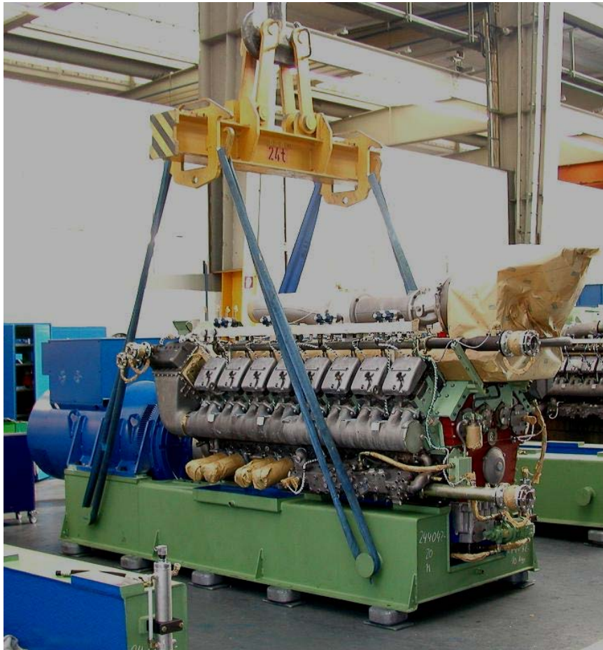
Fig. 18.1 Lifting a genset
